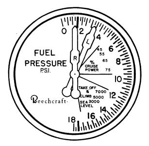
In the cruise power range the green sectors cover the fuel pressure required from 45% to 75% power. The lower edge of each sector is the normal-lean setting and the upper edge is the best power setting for that particular power range.
