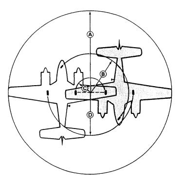
TURNING RADII ARE PREDICATED ON THE USE OF PAR-TIAL BRAKING ACTION AND DIFFERENTIAL POWER.
